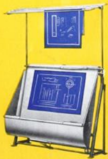
Every Penn "Senior" Sheet Washer has both spray pipe and drain pipe so that prints are washed with a continuous flow of clear, running water. Drain pipe is equipped with reversible strainer plug so that trough may be used as a bath tray when desired.
